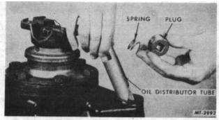
Fig. 2 Removal of Plug, Spring and Oil Distributor
