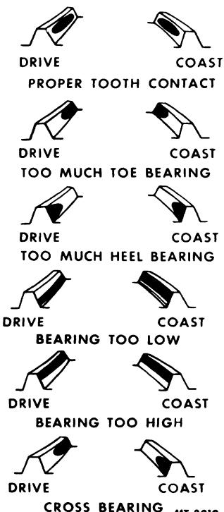
Fig. 35 Tooth-Contact Impressions
