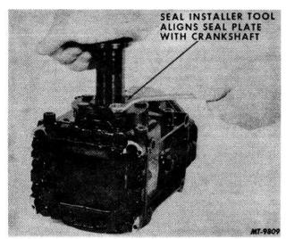
Fig. 33. Installing Seal Plate
