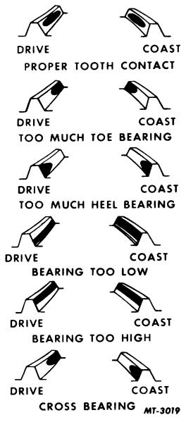
Fig. 20 Tooth Contact Impressions
