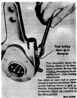
Fig. 2. Slack Adjuster Locking Sleeve on Adjusting Nut
