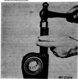
Fig. 20 Installing Worm Seal
