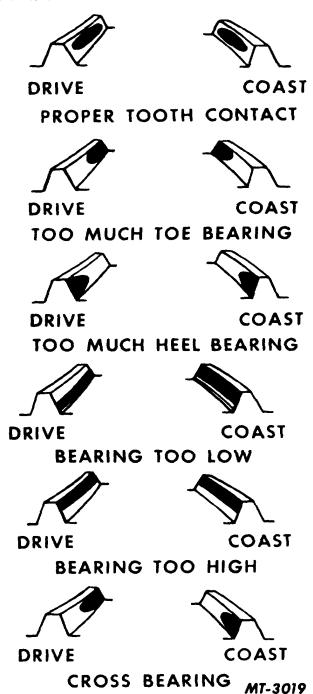
Fig. 38 Tooth Contact Impressions.
