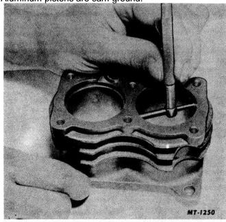
Fig. 6 Measuring Cylinder Bore Diameter
