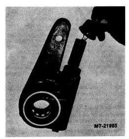
Fig. 10 Removing Actuator and Adjusting Sleeve Assembly
