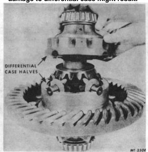
Fig. 13 Separating Differential Case Halves
