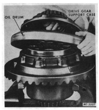
Fig. 18 Removing Support Case and Oil Drum.
