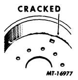
Fig. 6 Cracked Drum
