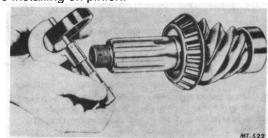
Fig. 23 Measuring Spacer Thickness
