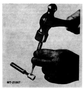
Fig. 13 Removing Piston from Actuator Rod
