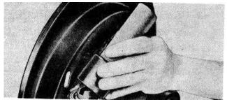
Driver must be centered over seal retainer to prevent damage to seal assembly.
