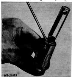
Fig. 21 Installing Original Design Piston Retaining Ring
