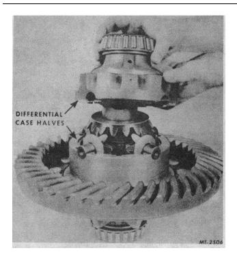
Fig. 17 Separating Differential Case Halves
