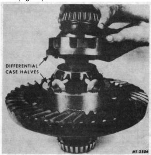
Fig. 17 Separating Diff Case Halves
