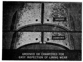
For visual inspection of brake lining wear, the linings of the Stopmaster II can be grooved on the side, as shown, as customer option. Also, as an option, the lining could be chamfered on the 4 inner corners, as shown.
