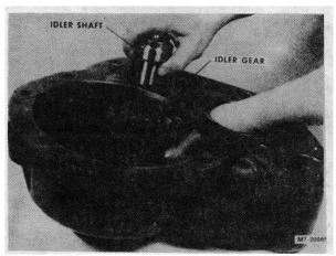
Fig. 13 Removing Idler Shaft and Gear
