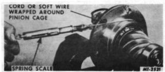
Fig. 27 Measuring Pinion Bearing Preload.
