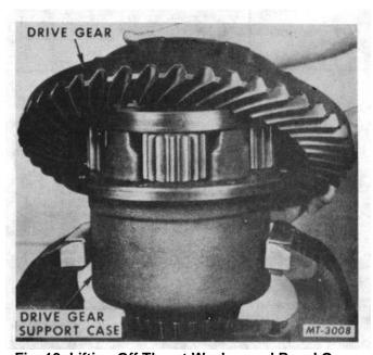
Fig. 19 Lifting Off Thrust Washer and Bevel Gear.
