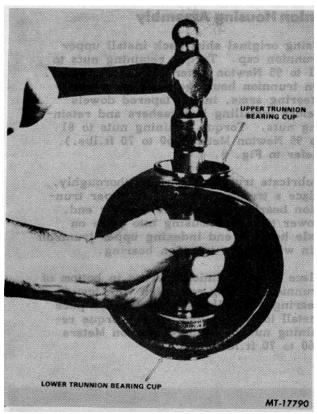
Fig. 14 Removing Trunnion Bearing Cup
