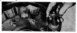
b. Coat adjusting bolt threads with grease and turn bolt into the adjusting plunger by working it through the hole in the outer seal flap, being careful not to pinch the seal on the threads. Turn adjusting bolt in just short of the seal. <a href="DO NOT">DO NOT</a> bottom bolt on the seal.
