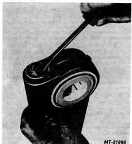
Fig. 14 Removing Worm Grease Seal
