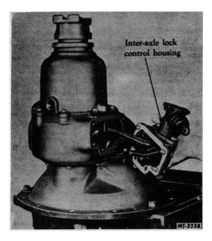
Fig. 4. Removing Inter-Axle Lock Control Assembly.
