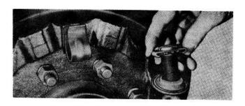
f. Coat adjusting bolt threads with grease and thread it into the sleeve after working it through the seal flap hole, being careful not to pinch the seal on the threads. Turn bolt in to just short of the seal. DO NOT bottom it on the seal.
