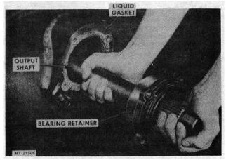
Fig. 50. Installing Output Shaft
