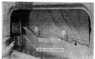
Fig. 12 Removing Rear Run Channel
