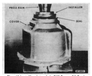
Fig. 42 Installing Inter-Axle Diff Cover Oil Seal
