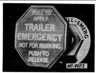
Fig. 3 Two-Way Control Valve (Push-Pull Type)
