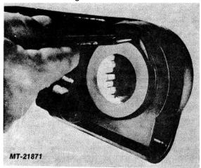
Fig. 17 Installing Seal on Gear Groove
