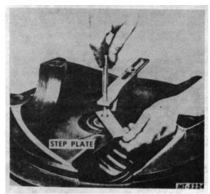
Fig. 17 Installing Step Plate
