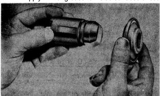
2. On <u>anchor (solid) plungers</u>--inspect nose for burrs. Mask brake shoe web slot in the plunger nose with masking tape to protect seal.
