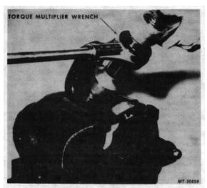
Fig. 43 Tightening Companion Flange Nut
