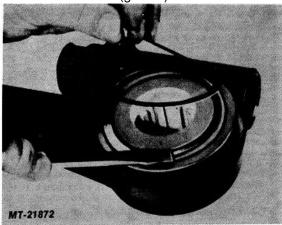
Fig. 18 Install Gear Retaining Rings
