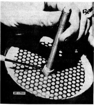
Fig. 14 Installing Second Perforated Plate
