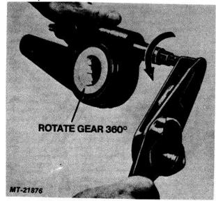
Fig. 23 Torque Check Slack Adjuster
