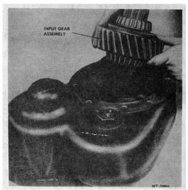
Fig. 12 Removing Input Gear Assembly
