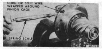
Fig. 22 Measuring Pinion Bearing Preload
