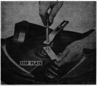
Fig. 30 Installing Step Plate
