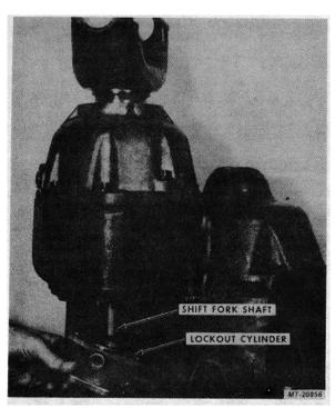
Fig. 3 Removing Inter-Axle Lockout Cylinder Assembly
