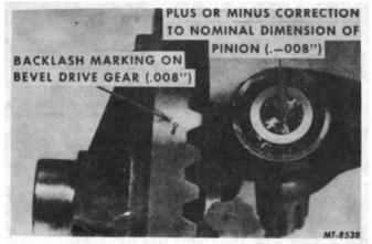
Fig. 25 Location of Pinion Setting Markings
