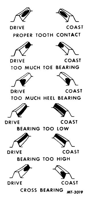
Fig. 24 Tooth Contact Impressions
