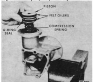
Fig. 12 Removing Piston Assembly.
