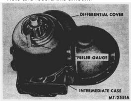
Fig. 43 Measuring Inter-Axle Differential End Play with Feeler Gauge.
