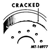
Fig. 6 Cracked Drum
