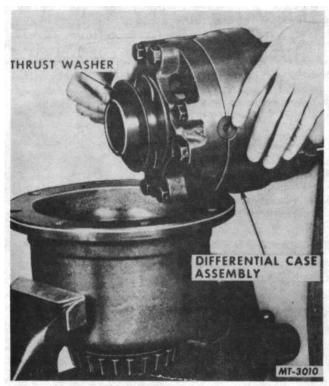
Fig. 21 Removal of Differential Assembly and Thrust Washer.
